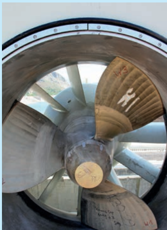
A matrix turbine waiting to be put to use
