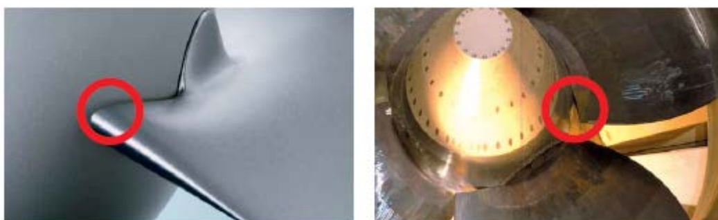
Figure 5-5: Adapted Kaplan turbine design (left) for increasing the fish survival rate by minimising the gap between the runner and the hub (compare to image on the right). Source: Hydropower Equipment Association
